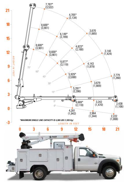
The 8051 is largest crane available to be mounted on a 19.5k GVW chassis. With 8,600 lbs of gross lifting capacity, 21 ft of full hydraulic reach, Auto II Speed and high speed planetary winch, the 8051 will be your jobsite workhorse.
