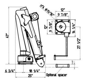
Power winch and wired remote control - standard on all models.
