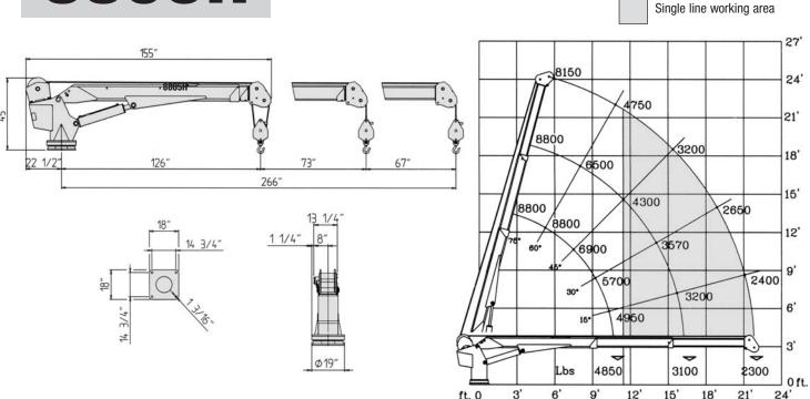
\* Cobra crane structures are designed for a normal working life of 12 - 15 years according to the DIN Standard 15018 (load classification H2-B3) with routine service and maintenance. Details available upon request.
