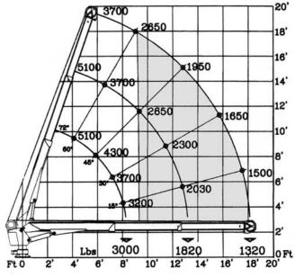
\* Cobra crane structures are designed for a normal working life of 12 - 15 years according to the DIN Standard 15018 (load classification H2-B3) with routine service and maintenance. Details available upon request.
