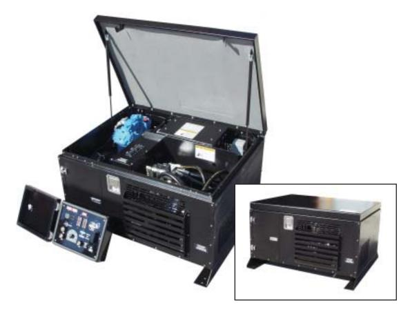
American Eagle has developed a new hydraulically driven power source for service trucks called the American Eagle Genesis. The truck mounted power source measures 48"x 36"x 29". It is hydraulically driven with a dedicated pump from the truck power take off. This power source requires 16GPM @ 3000 PSI to drive it with a maximum system pressure of 3500 psi. The unit is completely self-contained with a weather resistant remote control panel at the rear of the truck.
